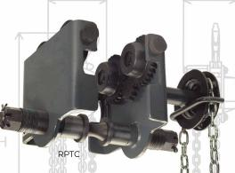
R&M trolleys are designed for both manual and electric operated hoists with a top hook suspension. Both the RPT push trolley and RPTC hand geared trolley are easily adjustable for a wide range of flange widths. Our RPTs are available in 1/4 - 5 ton (250 - 5000 kg) capacities, and the RPTCs are available in 1 - 10 ton (1000 - 10,000 kg) capacities.
